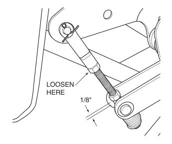
Figure 6-2. Brake Rod Adjustment
